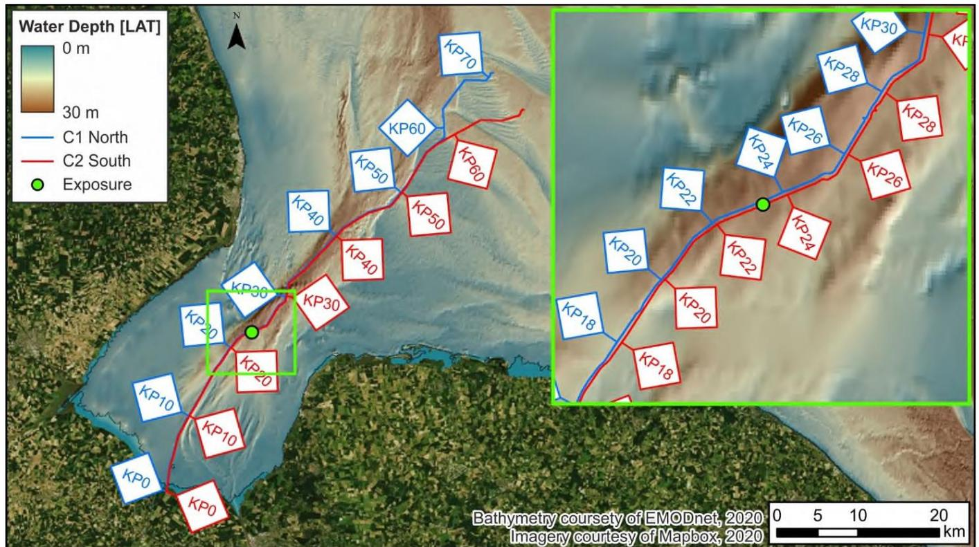
Figure 1: Location of possible cable exposure in relation to The Wash and Race Bank export cables
