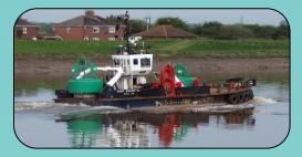
ST EDMUND – BUOY MAINTENANCE VESSEL. LOA 20 METRES, SPEED 9 KNOTS, CREW 6 MAX. CRANE SWL 6T @ 5M, 2T @ 12.5M.
