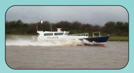
ST. ANN - PILOT CUTTER. LOA 13 METRES, SPEED 23 KNOTS. CREW 2 + 6 PASSENGERS MAX. CAT 2 WORKBOAT – 60NM FROM SAFE HAVEN.
