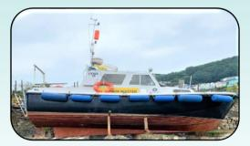
LYNX – HARBOUR PATROL & SURVEY LAUNCH. LOA 8.5 METRES, SPEED 10 KNOTS. CREW 4 MAX. CAT 3 WORKBOAT – 20NM FROM SAFE HAVEN.
