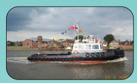
MT CONSERVATOR – STEEL HARBOUR TUG. LOA 16 METRES, SPEED 10 KNOTS, CREW 4 MAX. BOLLARD PULL 14 TONNES. CAT 2 WORKBOAT – 60NM FROM SAFE HAVEN.
