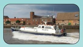
UNITED – PILOT CUTTER. LOA 12 METRES, SPEED 20 KNOTS. CREW 2 + 6 PASSENGERS MAX. CAT 3 WORKBOAT – 20NM FROM SAFE HAVEN.
