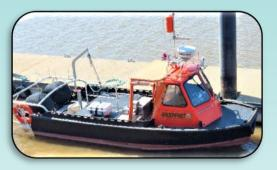
ARDENFAST – MULTI PURPOSE WORKBOAT. LOA 8 METRES, SPEED 25 KNOTS. CREW 4 MAX. CAT 3 WORKBOAT – 20NM FROM SAFE HAVEN.
